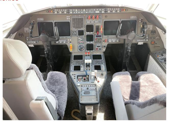
Collins EFIS /Pro Line 4 / Version 6.1 Flight System **High Frequency** Dual King KHF-950 Colins APS-4000 Autopilot w/ Coltech SELCAL Radar Collins TWR-850 **Traffic** Collins TTR-4100 (TCAS II Dual Collins VHF-422C Comms w/ Change 7.1) (8.33 kHz spacing) **Terrain** Allied Signal Mk-V EGPWS (TAWS-A) Dual Collins VIR-432 (w/ FM Immunity) INS Dual Honeywell Laseref IV's Navs Dual Collins DME-442 Dual Collins FMS-6100 **DME FMS** ADF Dual Collins ADF-462 w/ GPS-4000S
